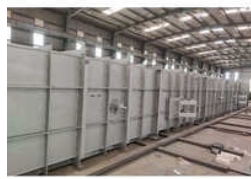
Mild Steel Furnace Casing
